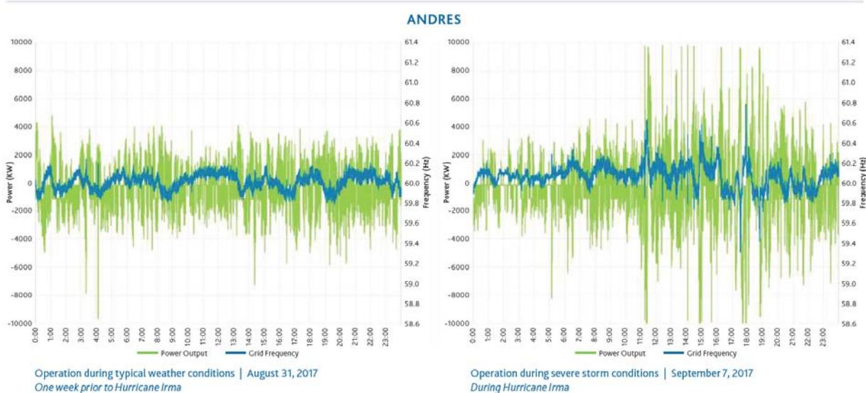
The graph above on the right shows that the measured frequency range increased significantly during the storm, moving from 59.3 to 60.8 Hz, and the energy storage system charged and discharged at maximum capacity (10 MW) on a number of occasions to quickly rebalance the system. The period of increased frequency disturbances lasted for more than 10 hours and the Andres energy storage array delivered 56.5% greater energy throughput than under typical operating conditions.
