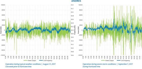
The graph above on the right shows that the measured frequency range increased significantly during the storm, moving from 59.3 to 60.8 Hz, and the energy storage system charged and discharged at maximum capacity (10 MW) on a number of occasions to quickly rebalance the system. The period of increased frequency disturbances lasted for more than 10 hours and the Andres energy storage array delivered 56.5% greater energy throughput than under typical operating conditions.
