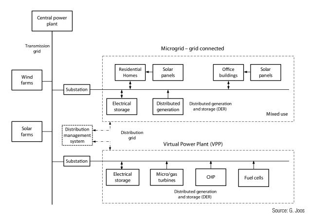
Figure 4 Aggregation of DER—microgrid and VPP
