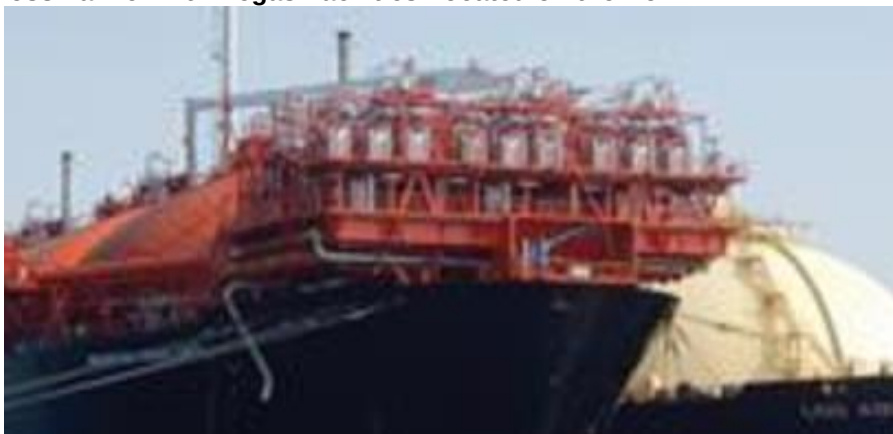
Figure 2.4 Moss Tanker with Regas Facilities Located on the Bow
