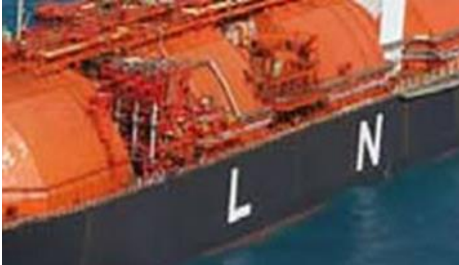
Figure 2.3 Moss Tanks with Regas Facilities Located Between the Tanks
