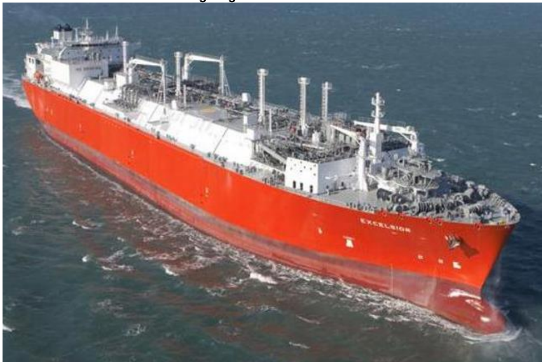
Figure 2.2 Membrane Tanks Showing Regas Facilities on the Deck
