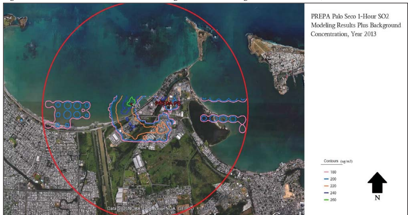
Figure 4: PREPA Palo Seco 1-Hour SO 2 Modeling Results Plus Background Concentration, Year 2013
