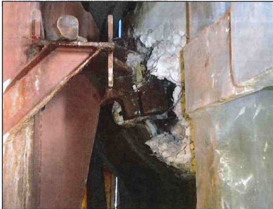
Photo 42 - U-6 Failed Control Valve Actuator Assembly Connection
