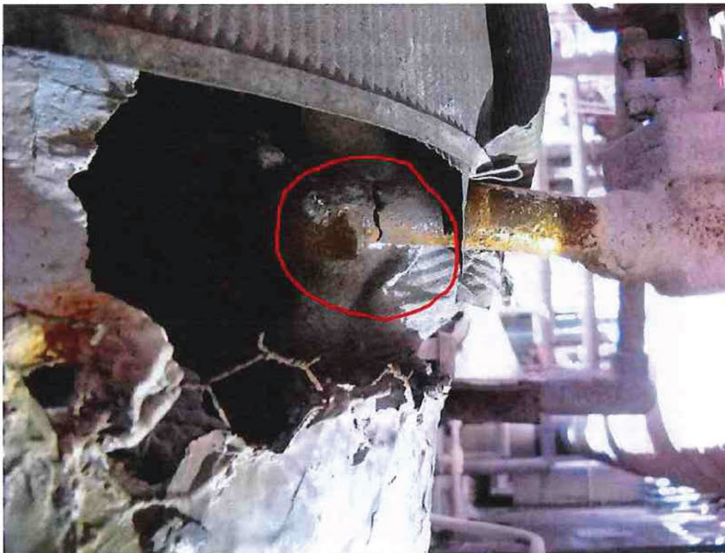
Photo 25 - U-6 Failed Pressure Tap
