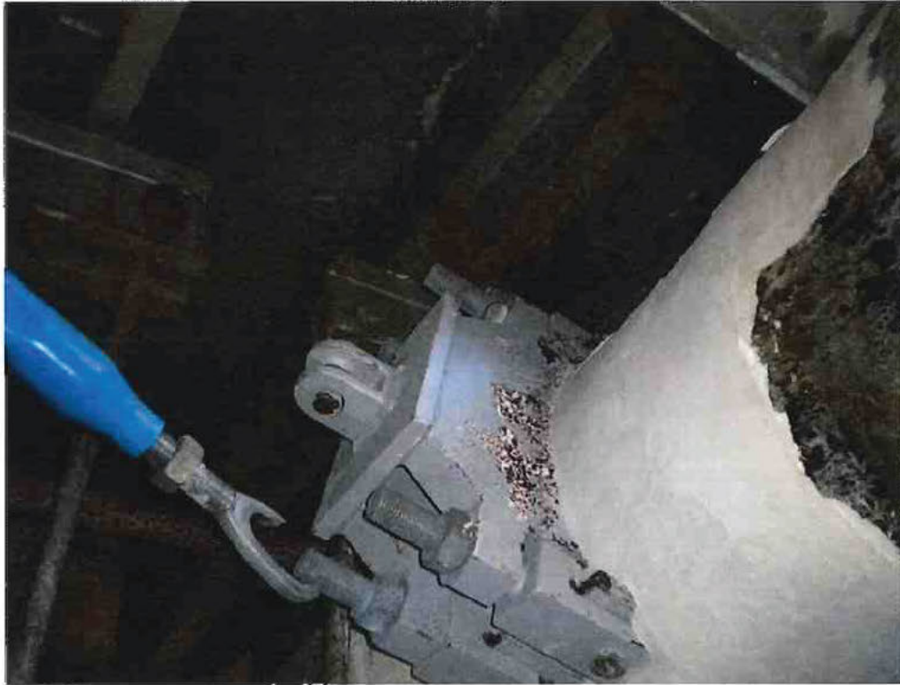
Photo 1 - U-5 Failed WEAR Restraint Rod End
