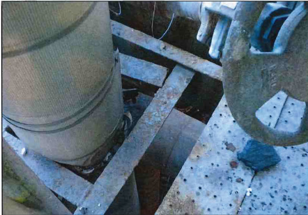
Photo 12 - U-5 Failed L-3 Boiler Feed Guide
