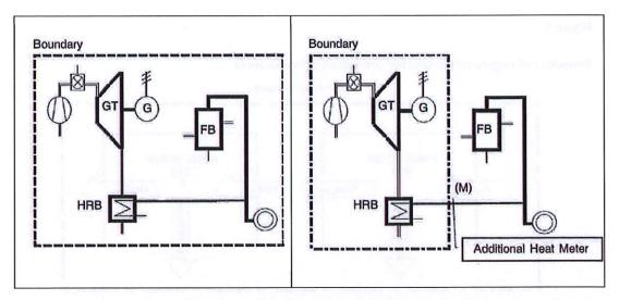
5. The secondary steam turbines (see Figure 4) must be included as part of the cogeneration unit. The electrical energy output of a secondary steam turbine forms part of the energy outputs from the cogeneration unit. The thermal energy required to produce these additional electrical energy outputs has to be excluded from the useful heat output of the cogeneration unit as a whole.
