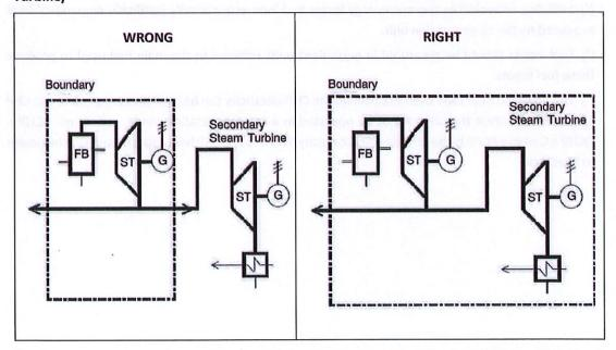
6. Where prime movers (i.e. engine or turbine) are connected in series (where the heat from one prime mover is converted to steam to supply a steam turbine), the prime movers cannot be considered separately, even if the steam turbine is located on a different site (see Figure 5).
