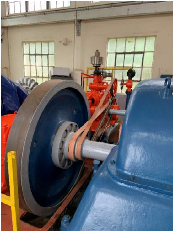
Photo 9-1 Río Blanco Flywheel, Belt Connections
