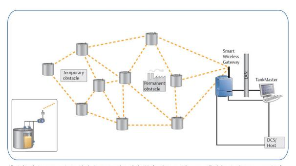
All wireless devices communicate with the host system through the Wireless Gateway. A Rosemount Tank Gauging System can consist of both wirel and wireless networks.
