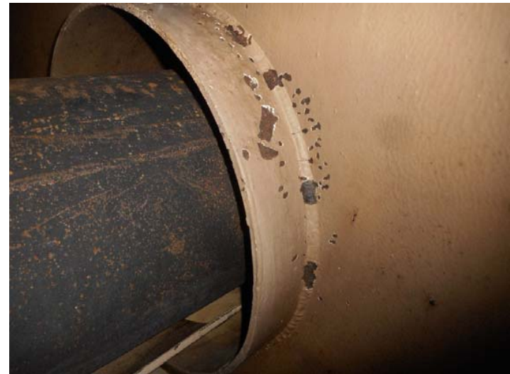
Coating Failures at N6
