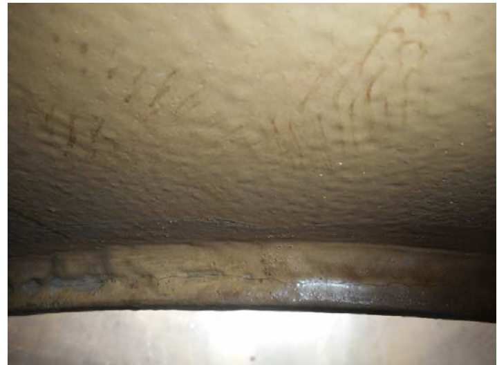
Coating Failures at Manway
