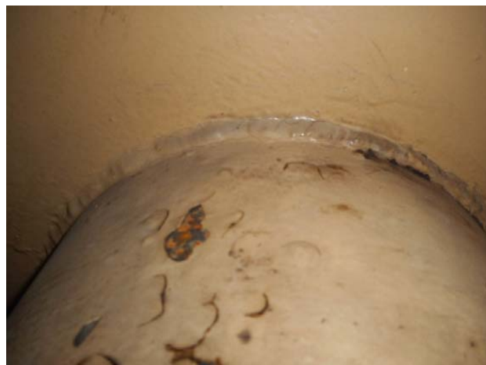
Coating Failures at N2
