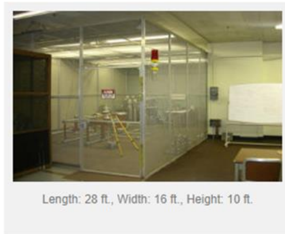
Figure 3- Faraday Cage for High-Voltage test Area
