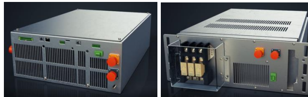
Figure 4. Compact bi-directional 100kW isolated DC/DC converter, and Compact bi-directional AC/DC converter.
