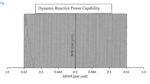
Figure 2 Reactive Power Capability Curve
