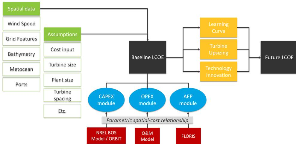
**Figure 28. The LCOE calculation process with NRWAL and reV**
