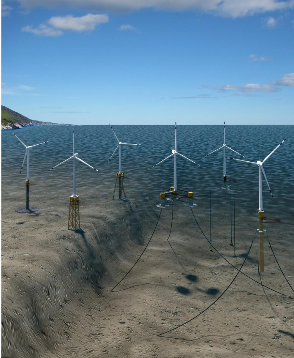
Figure 18. Example fixed-bottom and floating offshore wind substructures from left: monopile, jacket, twisted jacket, semisubmersible, tension-leg platform, and spar buoy. *Illustration by Joshua Bauer, NREL*
