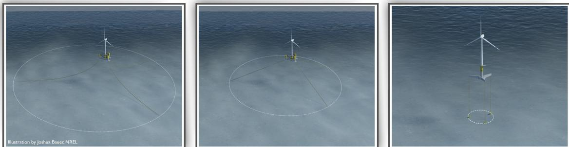
Figure 19. Floating offshore wind turbine mooring system footprint with mooring configurations from left: catenary, semitaught, and tension-leg platform. *Illustration by Joshua Bauer, NREL*
