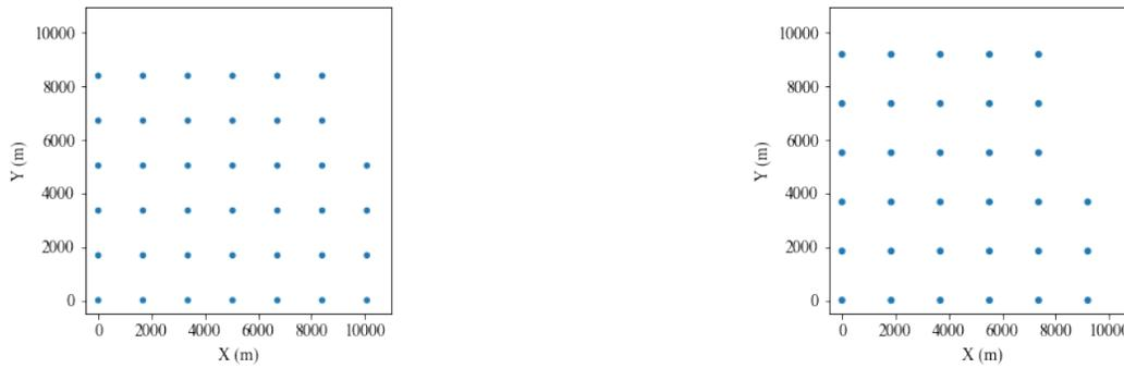
Figure 29. Assumed wind turbine layouts for (top) COD 2030 with 15-MW turbines and (bottom) COD 2035 with 18-MW turbines
