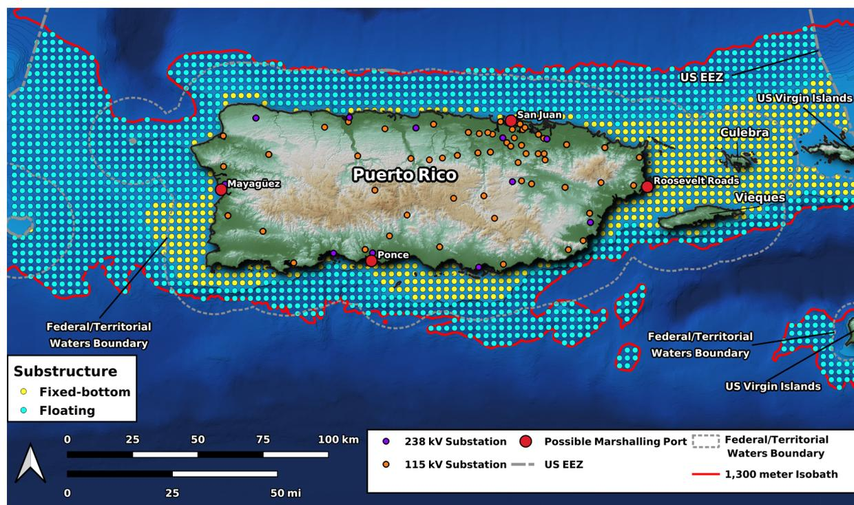
Figure 17. Fixed-bottom and floating wind resource points shown based on water depth. Fixed-bottom substructure are used in waters with depths between 5-m and 60-m, while floating substructures are used between 60-m and 1,300-m.
