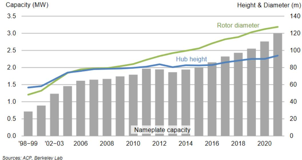
**Figure 14. Average wind turbine capacity, hub height, and rotor diameter for U.S. land-based wind projects over time. Image reproduced from Wiser et al. (2022) with permission**
