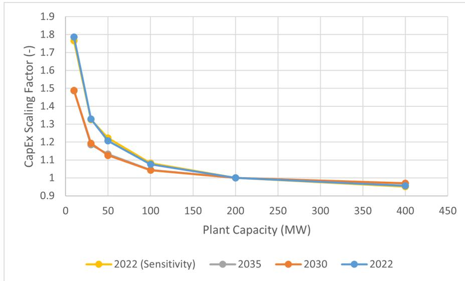
Figure 23. Land-based CapEx scaling factors for economies of plant size
