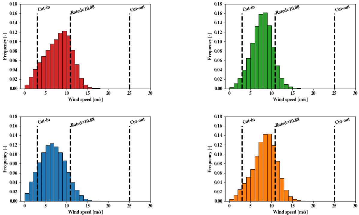
Figure 9. The 15-yr offshore wind speed distributions at a 160-m height for the (clockwise from top left) northwest, northeast, southeast, and west. Cut-in, rated, and cut-out wind speeds indicated from offshore wind turbines used in the modeling below (see Section 4).
