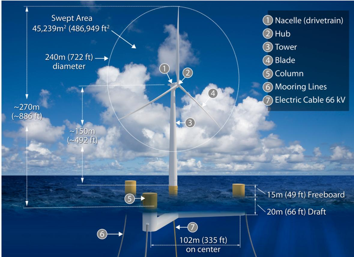
Figure 15. Representative offshore wind turbine technology assumptions for 2030. Illustration by Joshua Bauer, NREL
