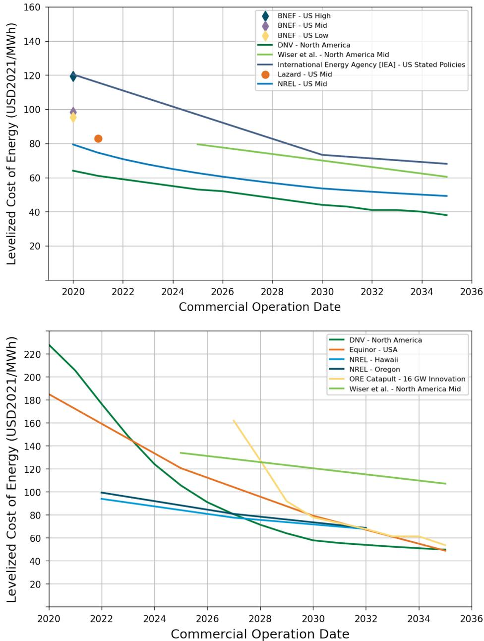
Figure 32. LCOE estimates from literature for fixed-bottom (top) and floating offshore wind (bottom). Images reproduced from Musial et al. (2022).
