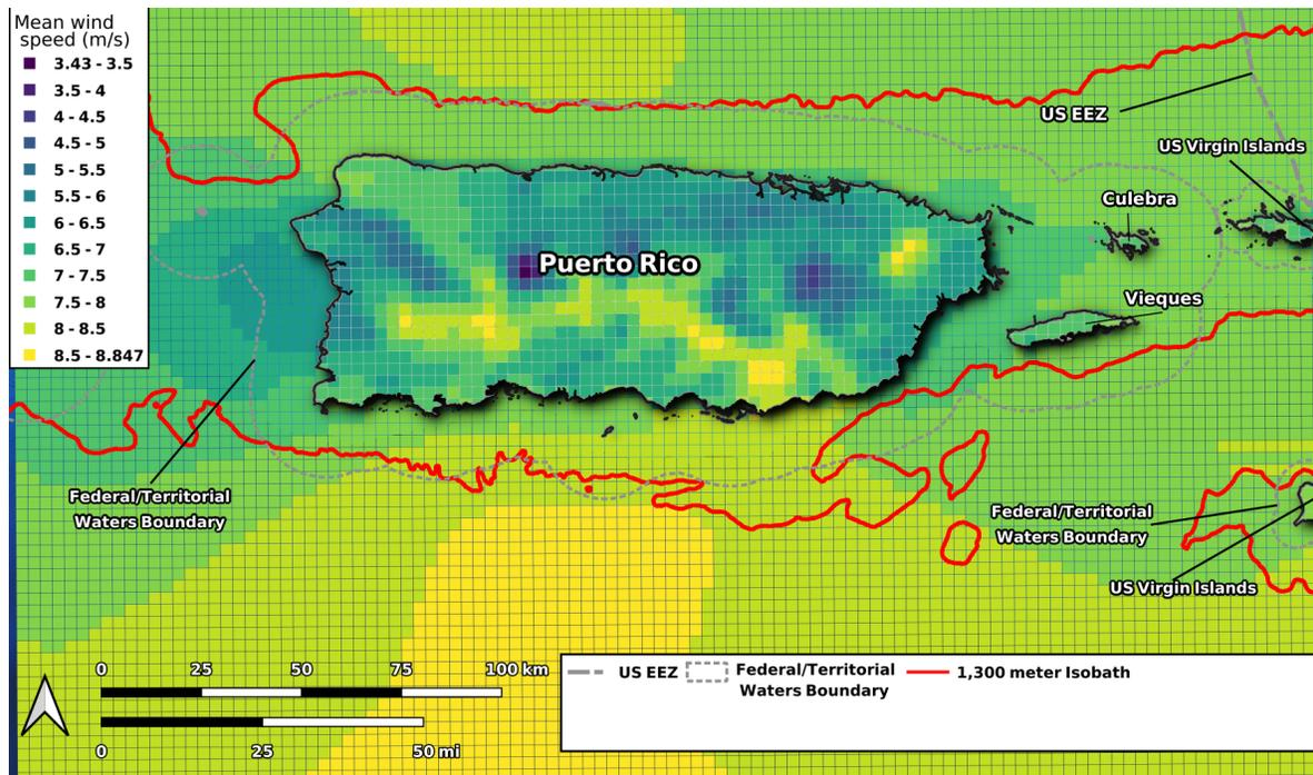
**Figure 2. Map of modeled 15-yr mean wind speeds (from PR20 data set) at 100 m for land-based wind and 160 m for offshore wind. The red line indicates the cost analysis domain defined primarily by water depths up to 1,300 m.**
