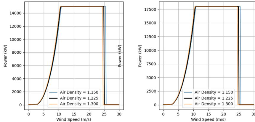
Figure 30. The 15-MW (left) and 18-MW (right) offshore wind power curves used for energy yield calculations based on the IEA 15-MW reference wind turbine (Gaertner et al. 2020)
