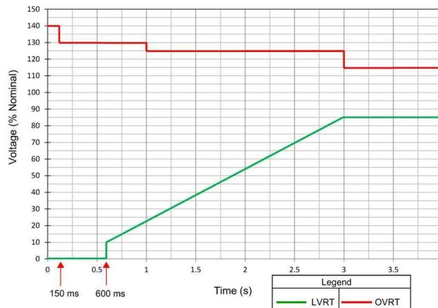
Figure 1 Voltage Ride-Through Requirements
