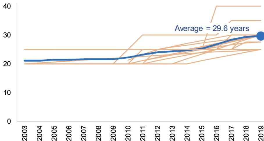
**Figure 26. Historical useful life of land-based wind turbines. Figure reproduced from Wiser and Bolinger (2019) with permission.**
