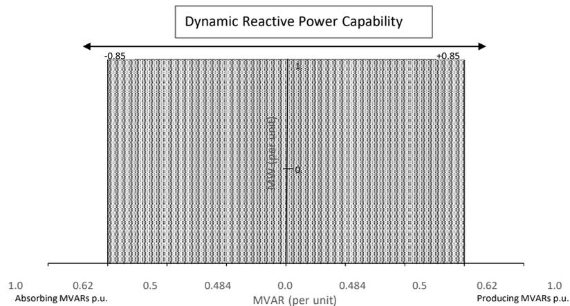
Figure 2 Reactive Power Capability Curve
