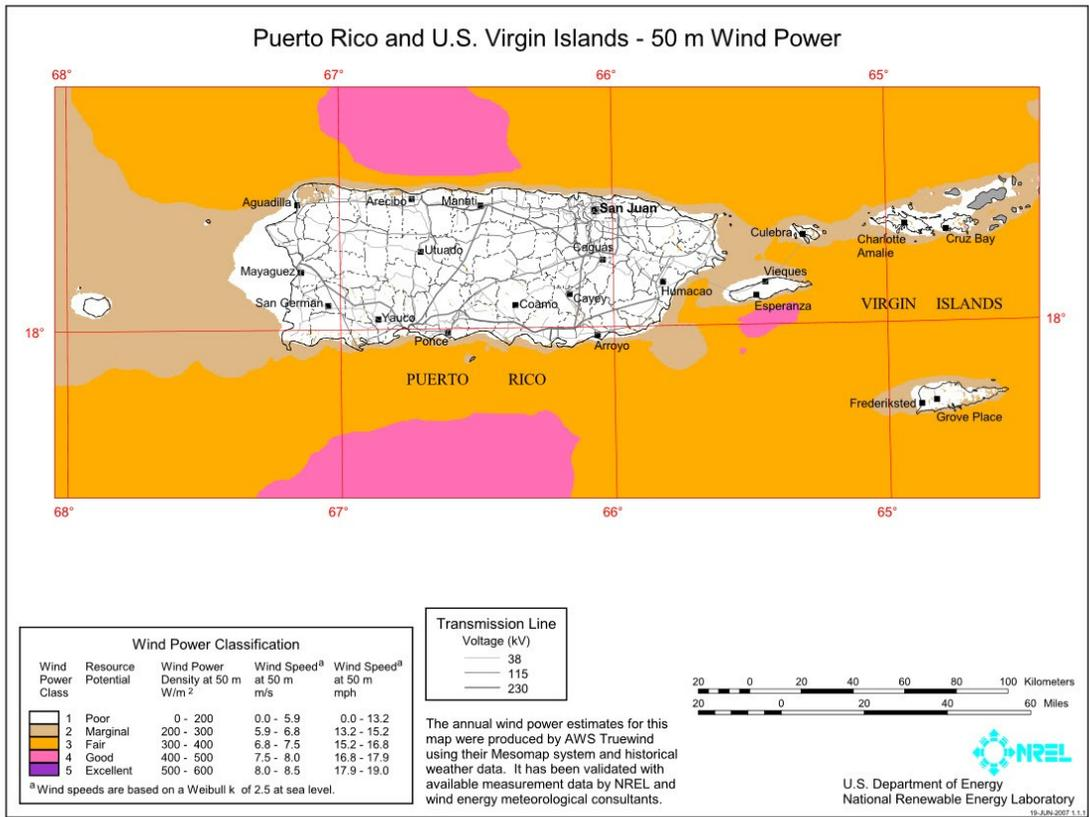
**Figure 3. Map of AWS Truepower data set mean wind speeds at 50 m offshore Puerto Rico and the U.S. Virgin Islands. Map previously produced by NREL (National Renewable Energy Laboratory 2007).**
