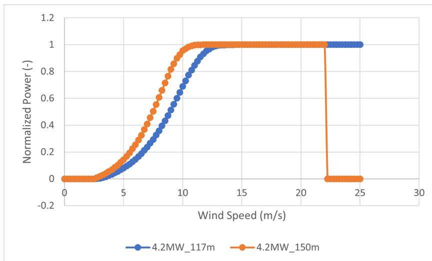
Figure 24. Land-based power curves used for energy yield calculations
