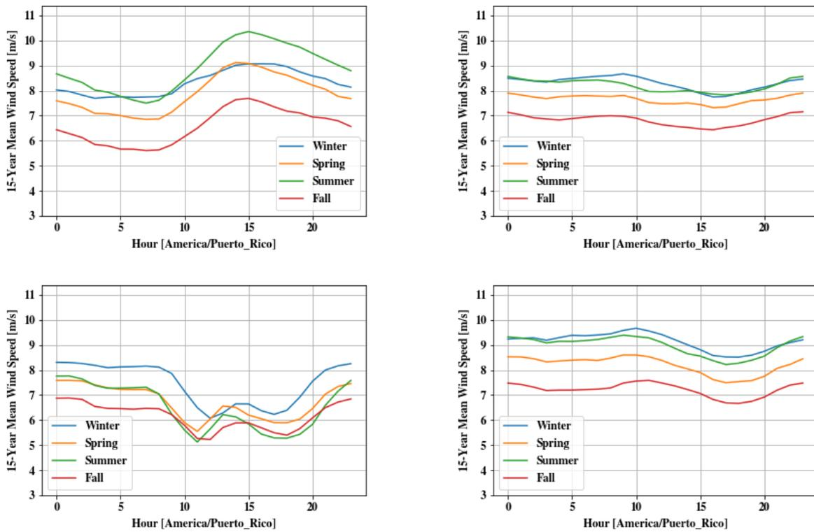
Figure 11. Diurnal profiles at 160 m offshore for the (clockwise from top left) northwest, northeast, southeast, and west
