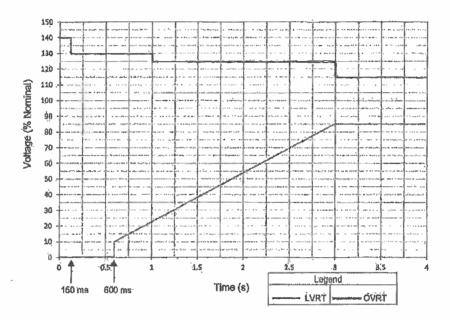
Figure 1 Voltage Ride-Through Requirements
