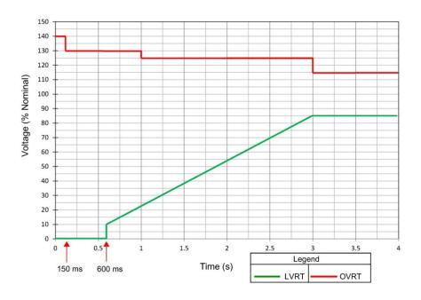
Figure 1 Voltage Ride-Through Requirements
