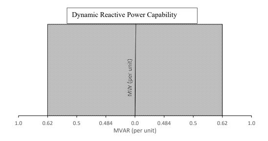
Figure 2 Reactive Power Capability Curve
