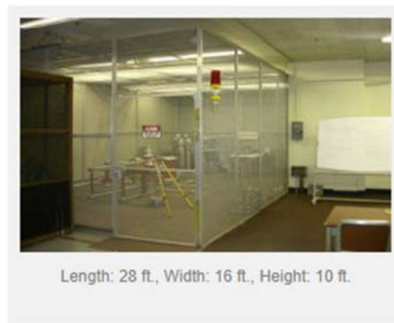
Figure 3- Faraday Cage for High-Voltage test Area
