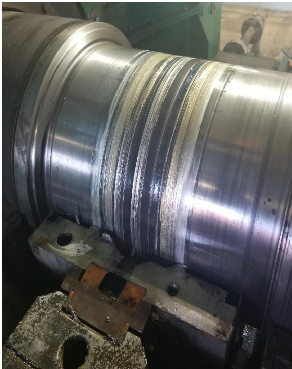
Steam Turbine Damaged Bearings Area Unit 5
