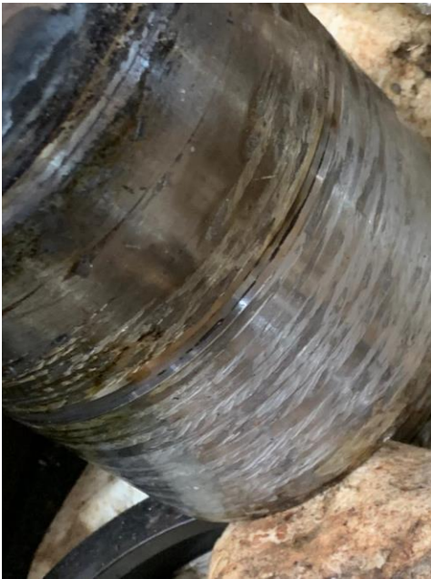
Damage Boiler Feed Water Pump Unit 2
