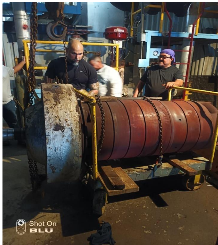
Damage Boiler Water Feed Pump 2-2
