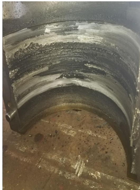
Steam Turbine Damaged Bearings Area Unit 5
