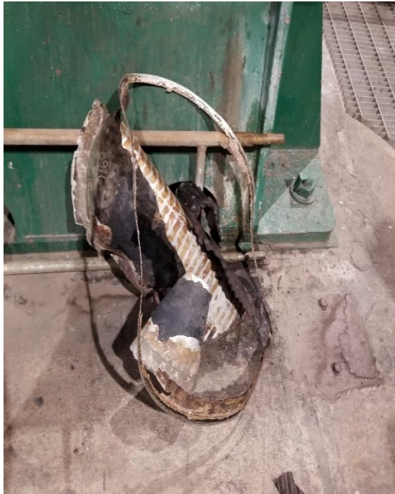
Steam Turbine Damage Area Unit 5 (Atmospheric Diaphragm Low Pressure Turbine)
