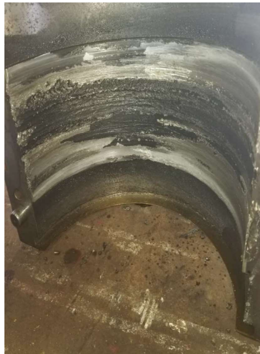
Steam Turbine Damaged Bearings Area Unit 5
