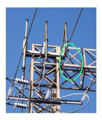
Figure 4 – Broken wedge connector on 38 kV side at San Juan generating plant
