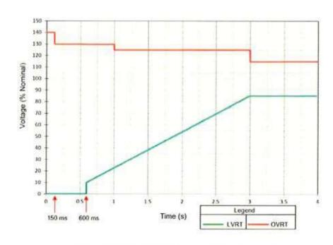
Figure 1 Voltage Ride-Through Requirements
