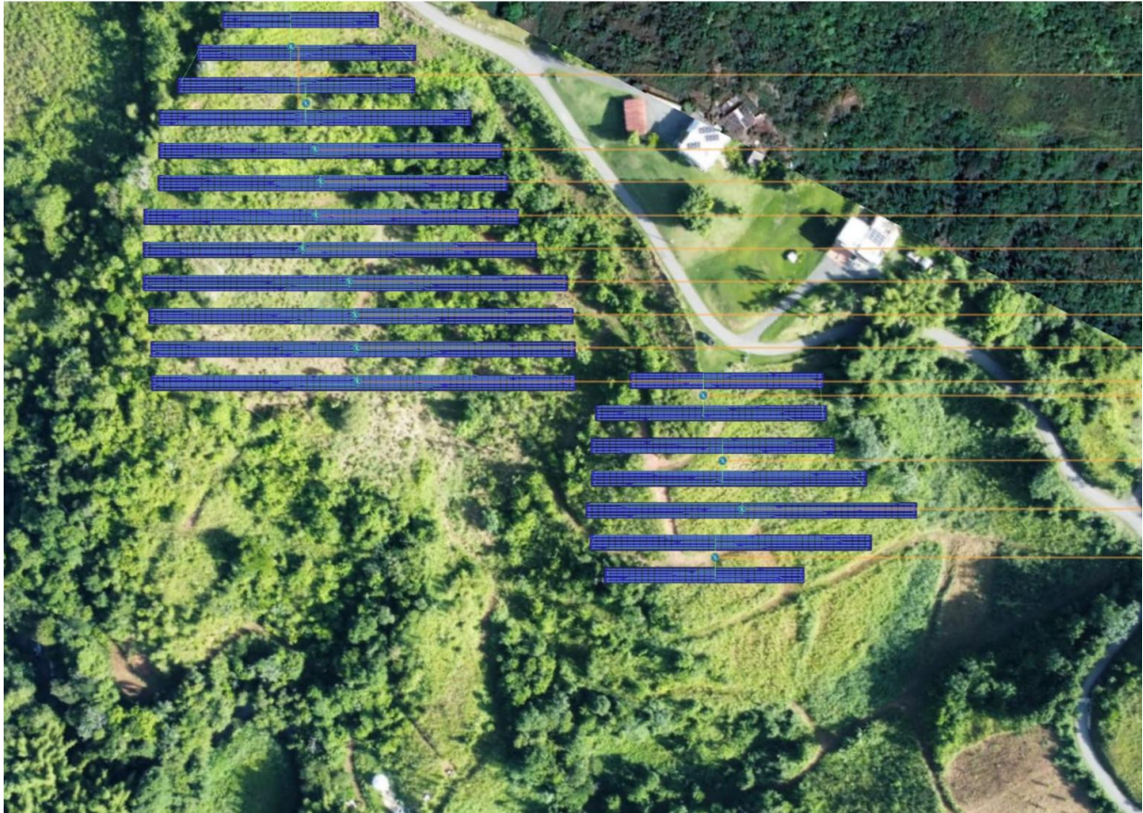
Figure 8: Close-up of conceptual layout of PV new solar energy system
