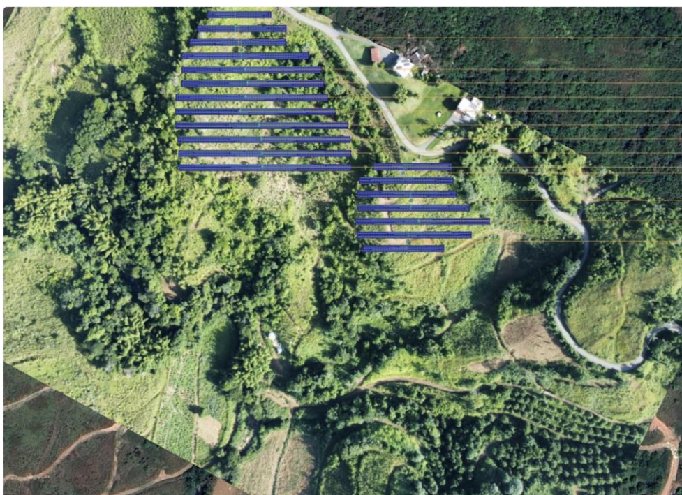
Figure 1: Conceptual Layout of PV new solar energy system
