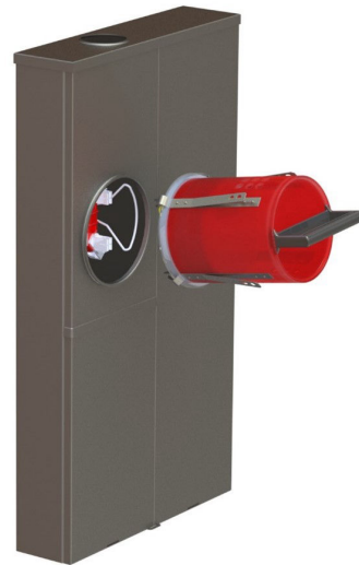
Pull the meter out of the meter socket
